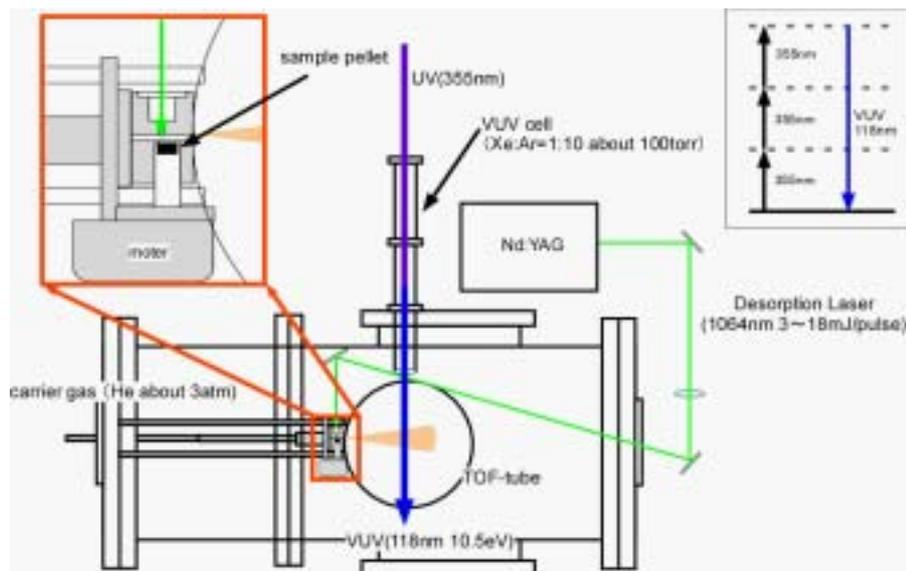
Fig. 1. Experimental setup of laser desorption / vacuum-ultraviolet photoionization mass spectrometry (LD/VUVPI MS), and the schematic diagram of VUV generation.
